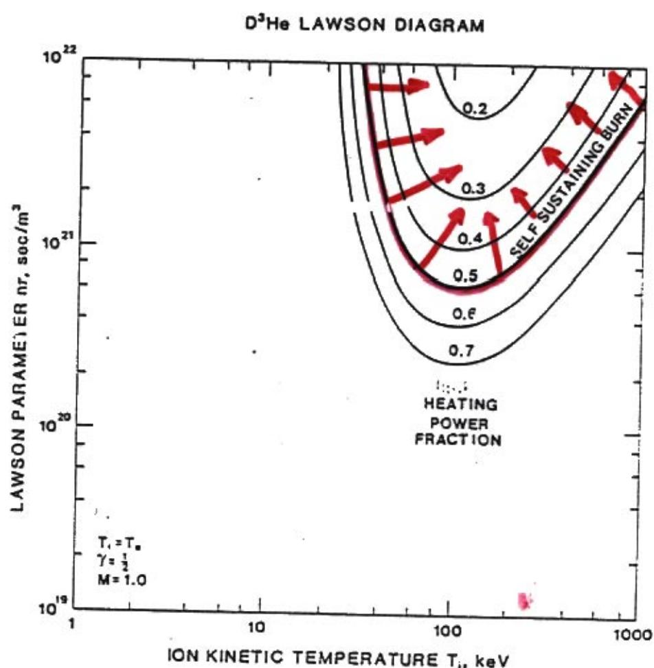
Lawson diagram for the D<sup>3</sup>-He fusion reaction. The required product of ion number density and particle containment time is plotted as a function of the ion kinetic temperature for several values of the heating power fraction,  $F_{hhj}$ .
