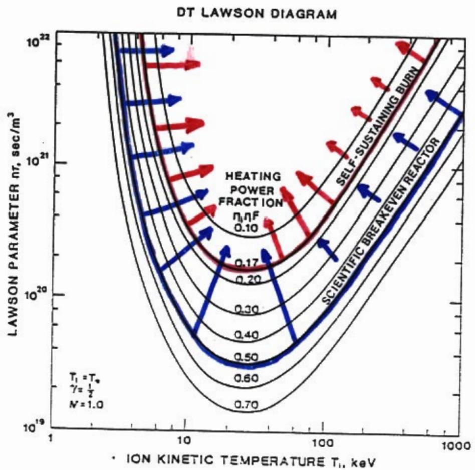
Lawson diagram for the DT fusion reaction. The parameters on the curves are the heating power fraction,  $F_{hh_i}$ . The required product of ion number density and particle containment time (Lawson parameter) is plotted as a function of the ion kinetic temperature.
